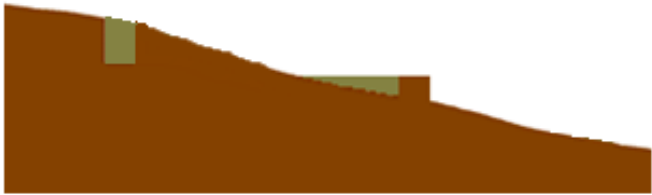
Pit Removal (Filling)
